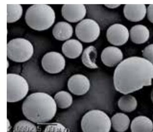
X-Bridge HILIC (13.5 nm, 5  $\mu\text{m}$ )
