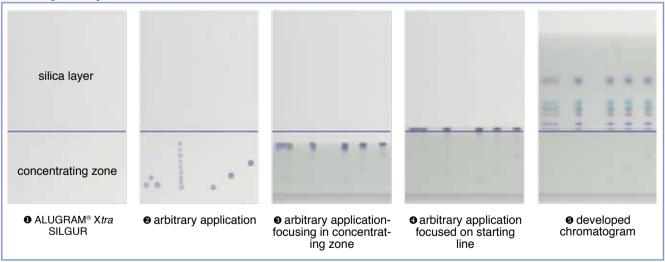
A valuable aid for manual application especially of large volumes of very dilute samples is the concentrating zone •, which consists of a chromatography inactive adsorbent (kieselguhr). The substances to be separated are concentrated to a narrow band in the concentrating zone •. The separation starts at the beginning of the chromatographically active adsorbent silica •.
