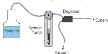
Gas bubbles are actively removed from a flowing liquid stream by vacuum via the PORIDEX membrane.
