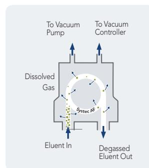
Dissolved gases are actively removed from a flowing liquid stream by vacuum via the Systec AF® membrane.
