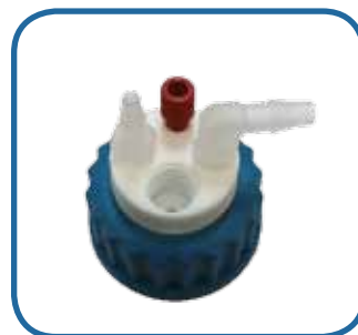
SW45-1-C-2L : 1 entry 1/8", 2 tube fittings and charcoal cartridge emplacement
