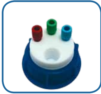
SWB-3-C : 3 entries 1/8" and charcoal cartridge emplacement
