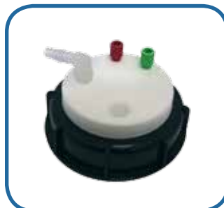
SW90-2-C-1L : 2 entries 1/8", a charcoal cartridge emplacement and 1 tube fitting
