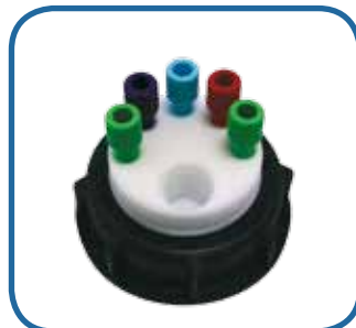
SW55-5-C : 5 entries 1/8" and a charcoal cartridge emplacement
