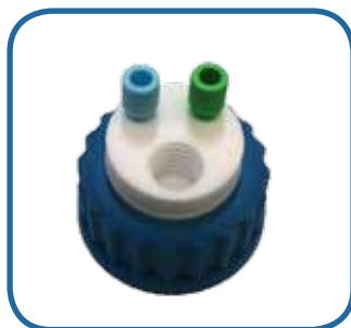
SW45-2-C : 2 entries 1/8" and charcoal cartridge emplacement
